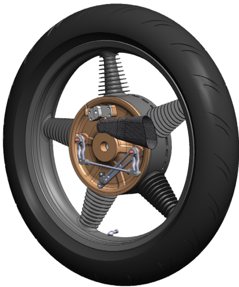
Monolithic Aluminum Wheel with Integrated Brake Drum CAD - 2023
