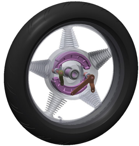
Monolithic Aluminum Wheel with Integrated Brake Drum CAD - 2023
